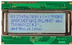
All parts come with a heater for -40°C to +85°C operation
