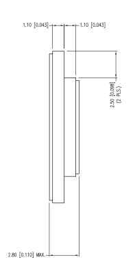
\*UNLESS OTHERWISE SPECIFIED TOLERANCES PER DECIMAL PRECISION ARE: X=±1 (±0.039), X.X=±0.5 (±0.020), X.XX=±0.25 (±0.010), X.XXX=±0.127 (±0.005). LEAD SIZE=±0.05 (±0.002), LEAD LENGTH=±0.75 (±0.030). MIN= +DECIMAL PRECISION MAX.= +0.00 (±0.001), X.XXX=±0.127 (±0.005). UNCONTROLLED DOCUMENT
