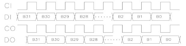
The serial command is transmitted with MSB first, DI is latched at the rising edge of CI clock. CO and DO are re-generated for the next SMD-LX1818RGBDWCTR LED. CO is inverted from CI. When 32 consecutive 0's are encountered, the next 1 is expected to start a 32-bit command, i.e., FLAG[2:0]=1xx. When FLAG[2:0]=1xx, then DIMMING,BLUE, GREEN and RED fields are latched respectively.
